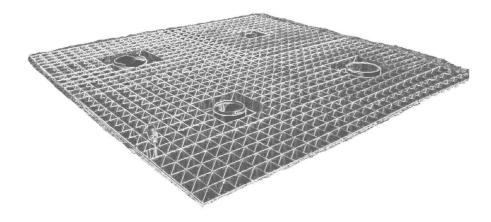
Figure 6 — Example of realization: 4-fold pit - Reference rain gauge pits of WMO Field Intercomparison of rain intensity gauges (Vigna di Valle, Italy, 2007)
