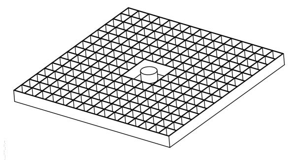
Figure 1 — General arrangement of raingauge pit and its grating as appearing at ground level
