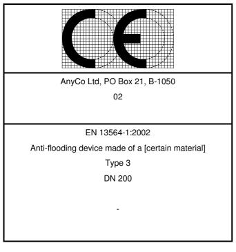
CE conformity marking, consisting of the "CE"-symbol given in Directive 93/68/EEC.
