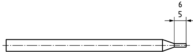
Figure 2 — Schematic view of pencil after sharpening
