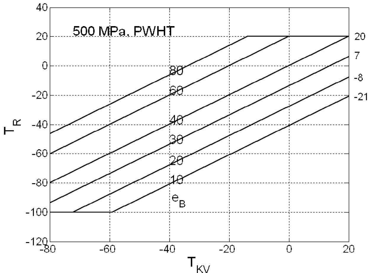
**Key** $T_R$  design reference temperature $T_{KV}$  material impact test temperature $e_B$  reference thickness
