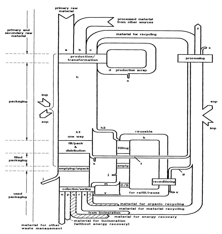
The size of flows do not correspond to the volume of the flows. Flows which are not possible with this material are shown hatched
