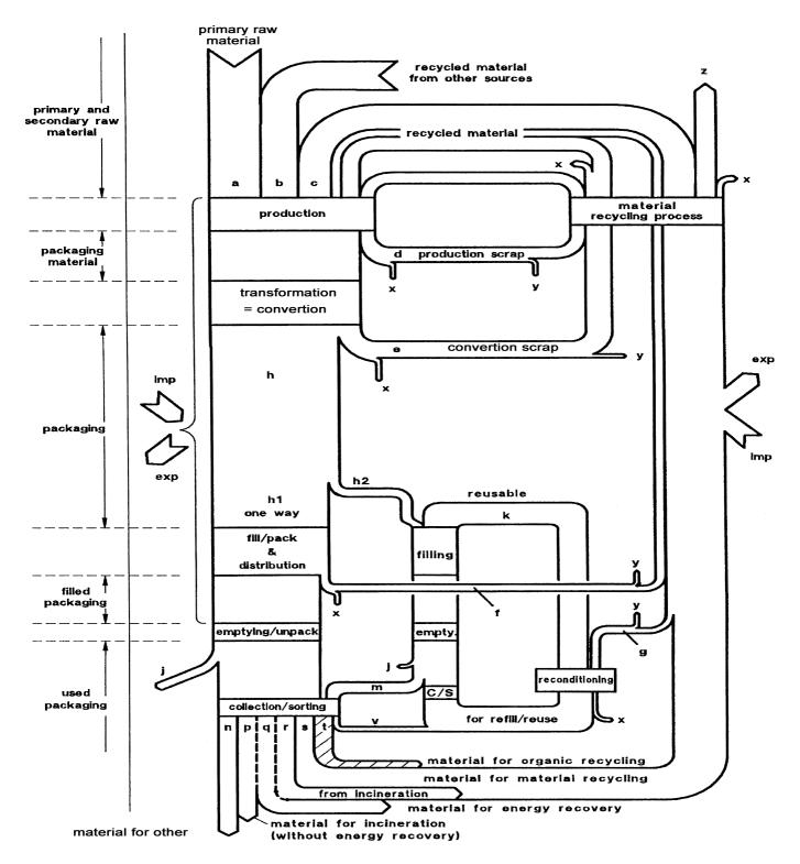
The size of flows do not correspond to the volume of the flows. Flows which are not possible with this material are shown hatched
