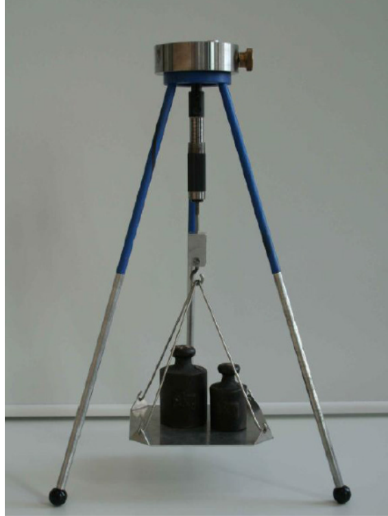
Figure H.1 — Suitable device for calibration of the small ball impact tester
