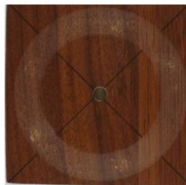
c) Excessive test: Wear-through has passed beyond the initial wear point
