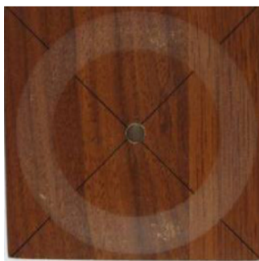
b) Correct test: Wear-through is evident in three quadrants
