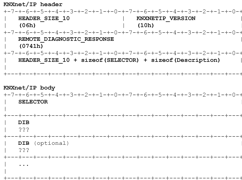
Figure 50 — REMOTE_DIAGNOSTIC_RESPONSE frame binary format
