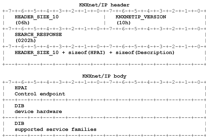
Figure 18 — SEARCH_RESPONSE frame binary format
