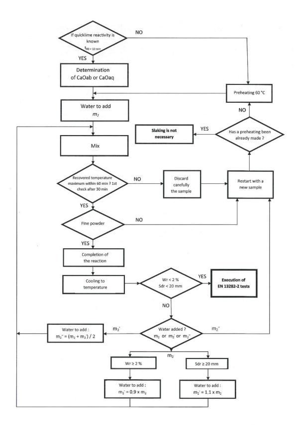
Figure A.1 — Flow chart for the slaking procedure
