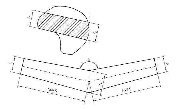
Figure 2 — Location of the zone of protection of head protectors
