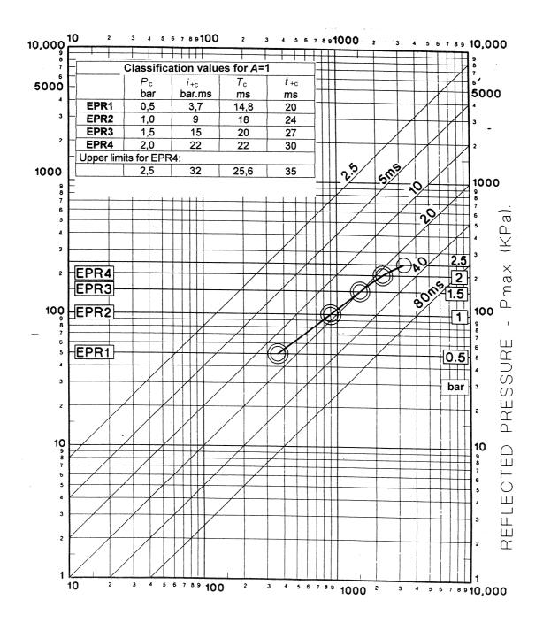
Reflected impulse  $i_+$  (kPa·ms), showing equivalent triangular durations  $t_{\blacktriangle}$  (ms).
