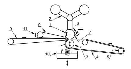
Figure 1b — Roller coating machine - Spreading belts configuration
