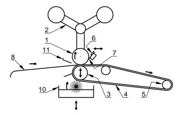
Figure 1a — Roller coating machine - Feeding-in table configuration
