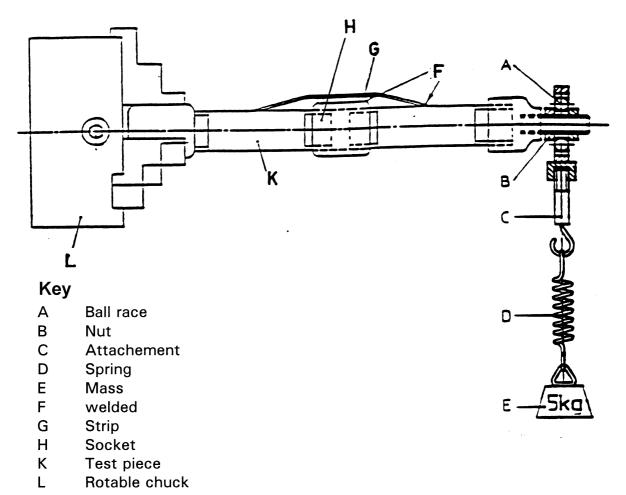
Figure 2 - Vibration rig
