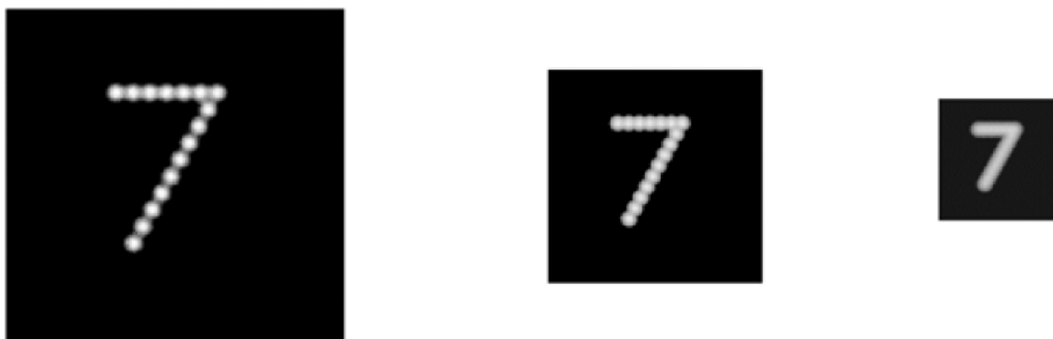
Figure M.1 — A legend seen at short (left), longer (centre), and very long distance (right)
