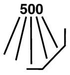
Figure 1 — Symbol to be used for marking containing the number of test cycles (500 in this example) corresponding to the test result
