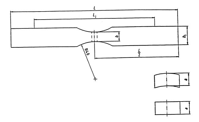
Figure 1 - Low temperature tensile test specimen
