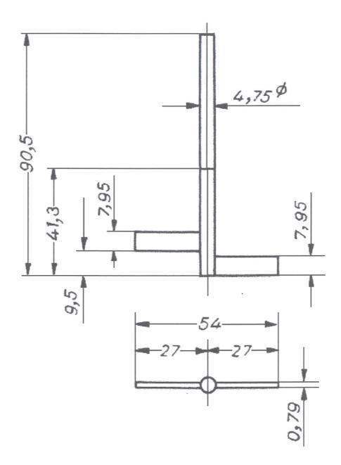
Figure G.2 – Paddle-type rotor in mm
