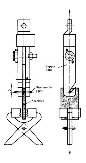
Figure 1 - Example of clamping device
