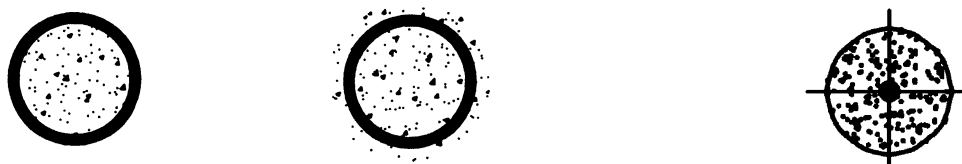
a) Examples of cross sections of prefabricated concrete piles
