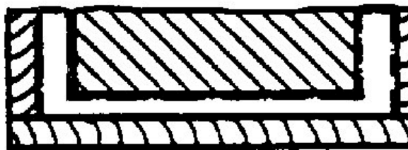
Figure 5 — Sample cut from a surfacing lying on a plank and tied on firmly
