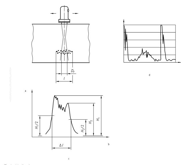
Group of indications, mainly non-resolvable individual indication. Dimension of indication range equal to or larger than sound-beam diameter  $D_{\rm F}$ .
