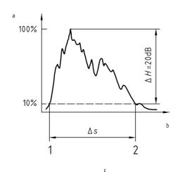
Individual echo with pronounced echo dynamics only in through-wall direction (travelling indication), or both in through-wall direction and parallel to the test surface:
