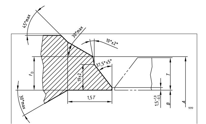
Figure 3 — Single-V butt weld end connection with V root to pipe of wall thickness T > 22 mm
