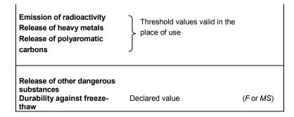
Figure ZA.2 — Example of CE marking information for aggregates for concrete under system 4
