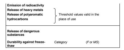
Figure ZA.1 — Example of CE marking information for aggregates for concrete under system 2+
