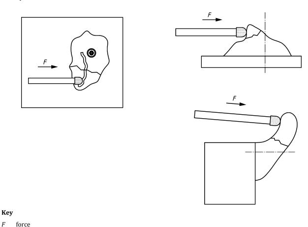
Figure A.1 — Setup (3 examples) for testing the structural integrity
