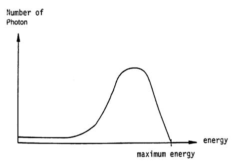
Figure 2 - Schematic shape of an X-ray spectrum after attenuation by a filter
