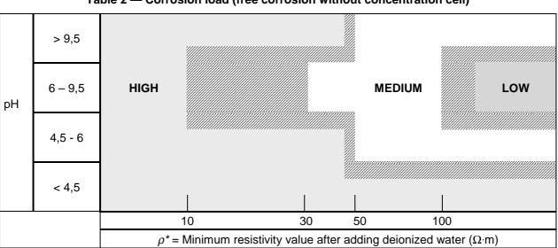
Table 2 — Corrosion load (free corrosion without concentration cell)
