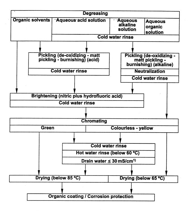
Figure A.1 — Treatment stages of the chromating of aluminium and aluminium alloys
