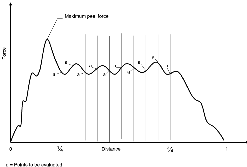
Figure 3 Graph for calculating the peel resistance (example)
