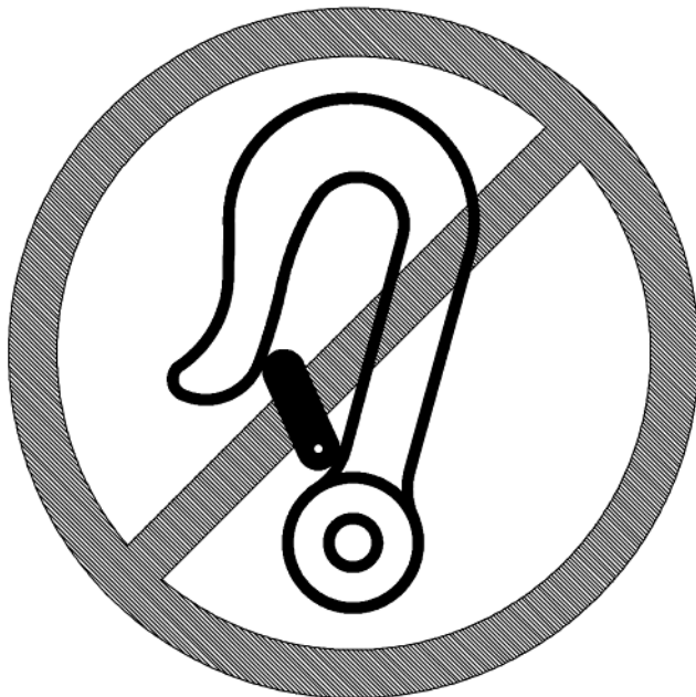
Figure 7 — Symbol for wheelchair not intended to be used as a seat in a motor vehicle
