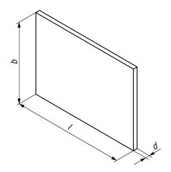
Figure 1 — Dimensions of a modular tile
