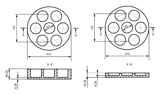
NOTE Adapt the dimensions of the holes according to the dimensions of the beakers available.
