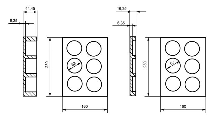
NOTE Adapt the dimensions of the holes according to the dimensions of the beakers available.
