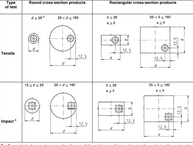
For products of a round cross-section, the axis of the notch is parallel to a diameter; for products with a rectangular cross-section, the axis of the notch is perpendicular to the greatest rolled surface.
