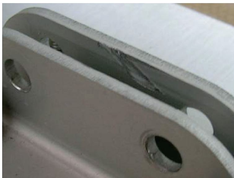
Figure A.22 — Example of a chafing finding
