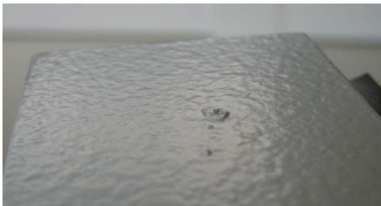
Figure A.38 — Example of a thin layer finding
