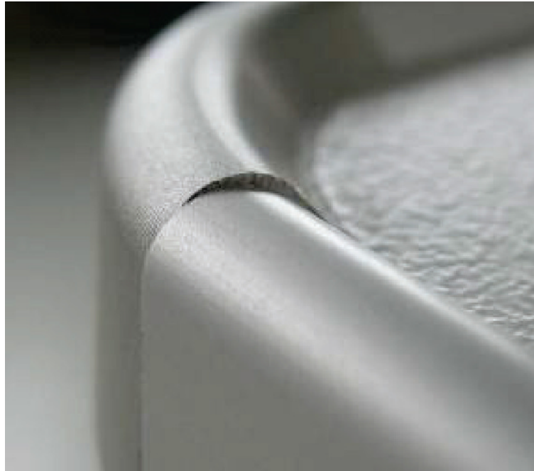
Figure A.13 — Example of an alignment finding
