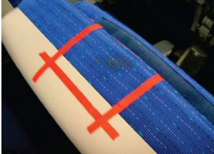
Figure A.28 — Example of a stain finding
