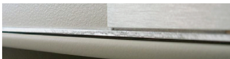
Figure A.23 — Example of a chafing finding
