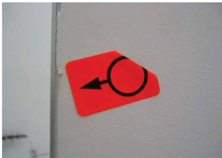
Figure A.18 — Example of an uneven edge finding
