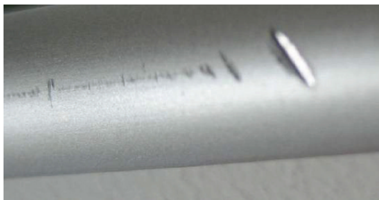
Figure A.25 — Example of a cut finding
