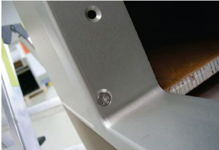
Figure A.32 — Example of a missing screw finding
