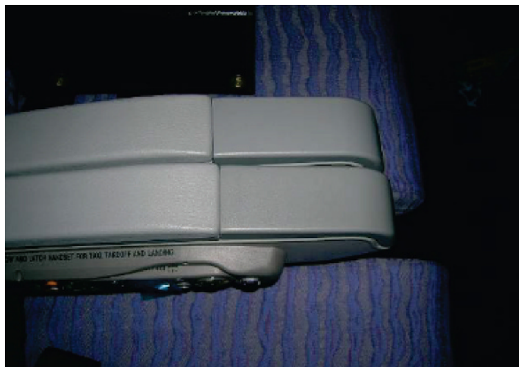
Figure A.14 — Example of a misalignment finding
