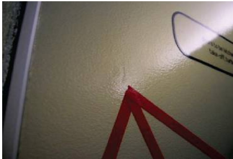
Figure A.17 — Example of a dent finding
