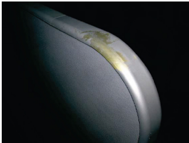
Figure A.20 — Example of a discolouration finding
