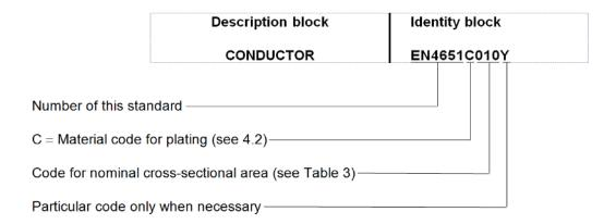
NOTE If necessary, the code I9005 shall be placed between the description block and the identity block.
