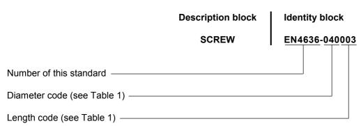
NOTE If necessary, the code 19005 shall be placed between the description block and the identity block.
