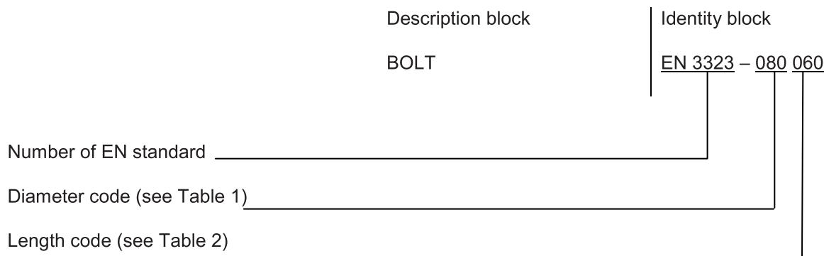
NOTE If necessary, the design code I 9005 may be placed between the description block and the identity block.
