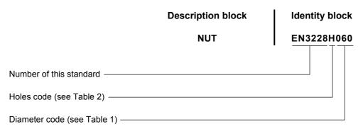
NOTE If necessary the originator code I9005 shall be placed between the description block and the identity block.
