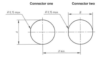
X min. value is calculated as follows: D/2 connector one + D/2 connector two (see Table 3 for value D).
