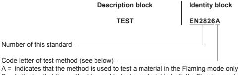
A = indicates that the method is used to test a material in the Flaming mode only.
