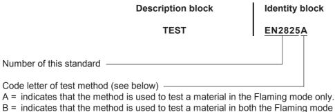
B = indicates that the method is used to test a material in both the Flaming mode and the Norm-Flaming mode.
