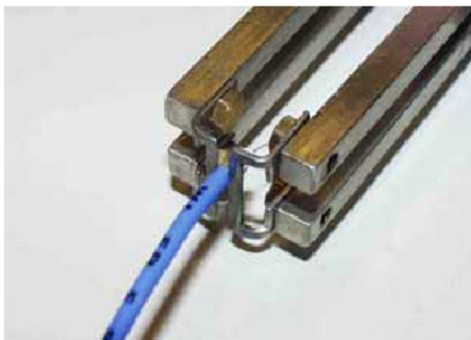
Figure D.1 — Stripping principle (rotating electrodes)
