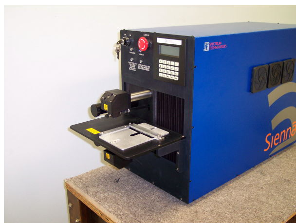
Figure C.2 — Example of laser stripping tool
