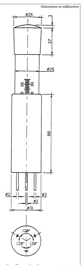
Figure 1 — Example of an apparatus to measure thickness by method B
