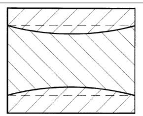
Figure 3 — Non-rigid specimens
