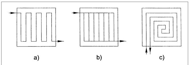
Figure 2 — Examples of schematic design of heating or cooling units in the case of external liquid supply
