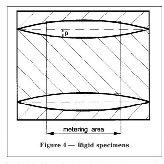
NOTE Table 2 shows that the required levels of flatness for both the specimen and apparatus surfaces are stringent, so that the use of contact sheets can be suggested even for specimens having a thermal resistance greater than  $0.3~\mathrm{m}^2\cdot\mathrm{K/W}.$
