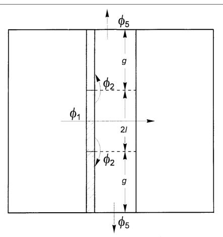
NOTE Heat flows at a rate  $\Phi_1$  through the metering area  $A = (2D)^2$ ; in the metering area the density of heat flow rate, q, is expected to be uniform;  $\Phi_2$  is an imbalance heat flow rate parallel to the specimen;  $\Phi_5$  is the transverse heat flow rate at the edge of the specimen; g is the guard width.
