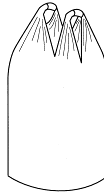
Lifting devices formed out of the walls
