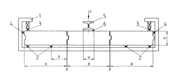
a = b – 2h  $\geq$  100 mm is the maximum permitted gap g is the maximum permitted gap
