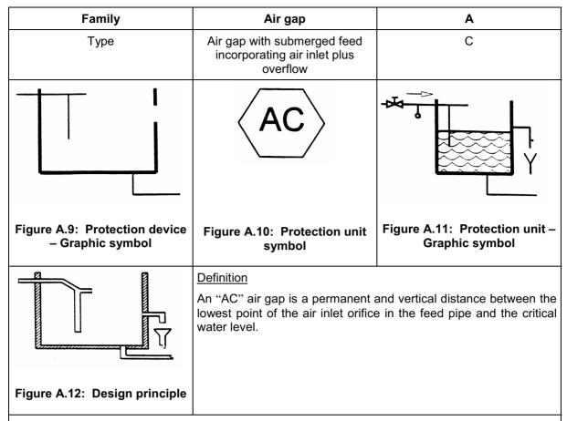
The protection device shall conform to the national standard transposing the European Standard as available.
