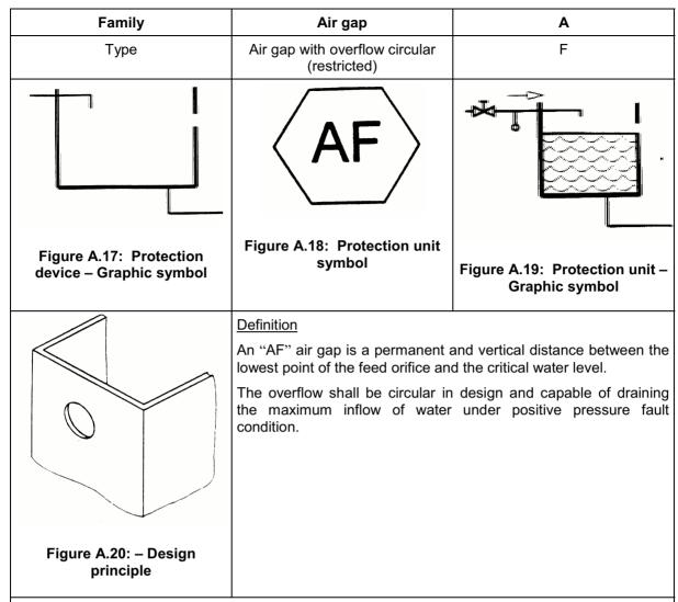
The protection device shall conform to the national standard transposing the European Standard as available.
