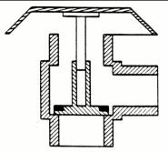
Mechanical device with an air inlet that is closed when water flows through it at or above atmospheric pressure, but that opens to admit air if there is a subatmospheric pressure at the water inlet or when flow stops, and closes so as to be watertight when the flow of water is resumed at normal pressure.
