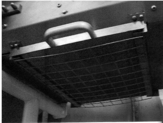
Figure 3 — Fixed mesh guard positioned below spillage tray
