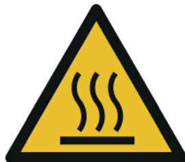
Figure 12 — Warning pictogram “Warning, hot surface”
