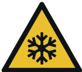
Figure 13 — Warning pictogram “Warning, cold surface”
