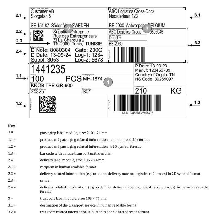
Figure A.12 — Example of the modularized multi industry transport label with three label modules in A5 format, horizontal orientation
