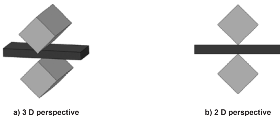
Figure F.1 — Principle of wedge penetration test
