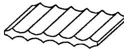
d) Grooved metal with or without a layer of additional gasket material (type ---/D)
